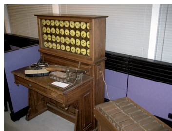
Punch card counting machine used for early census automation in the 1890s. Photo: Adam Schuster – Flickr: Proto IBM
